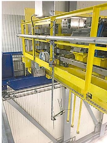
Fig. 1. Placement of the instrument on the Safe Trolley of MCS
